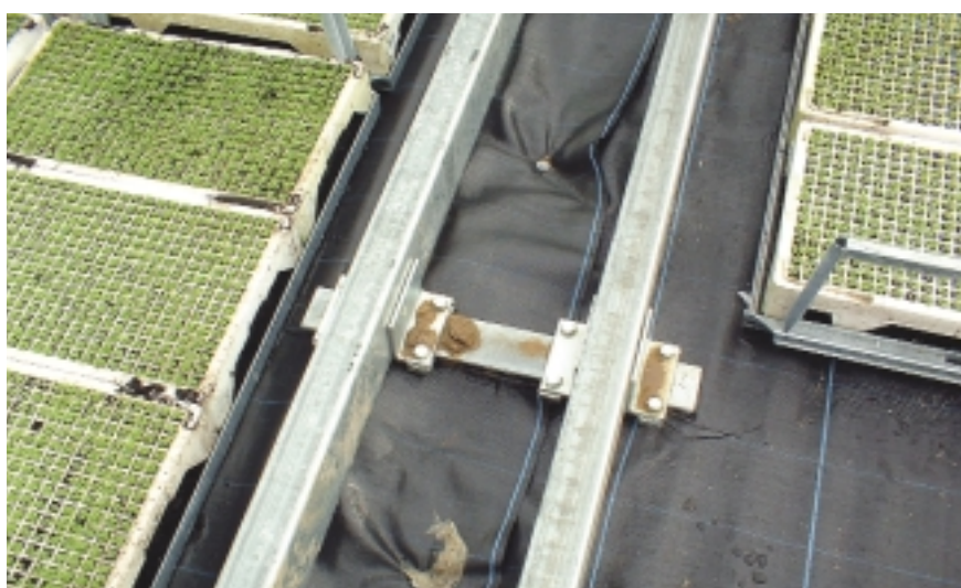
Above: Cranes are a more commonly used XY component in U.S. greenhouses. Below: Pick and place units can be designed to run on rails such as these, eliminating the need for concrete floors.
